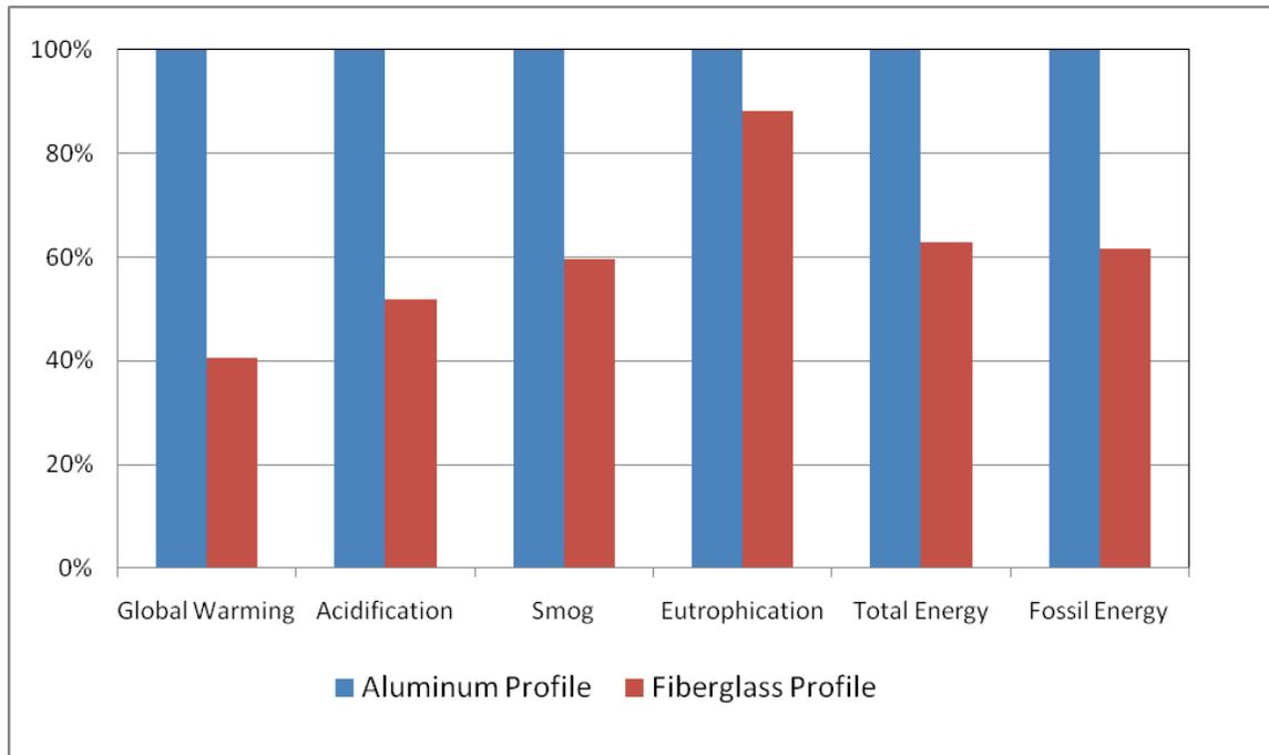
The results indicate a strong preference for the fiberglass mullion profile. Across each indicator measure the fiberglass mullion profile demonstrates a lower cradle-to-gate environmental impact. Depending on the impact indicator of interest, the fiberglass mullion results are between 40% to 90% of the aluminum mullion environmental burden results.
