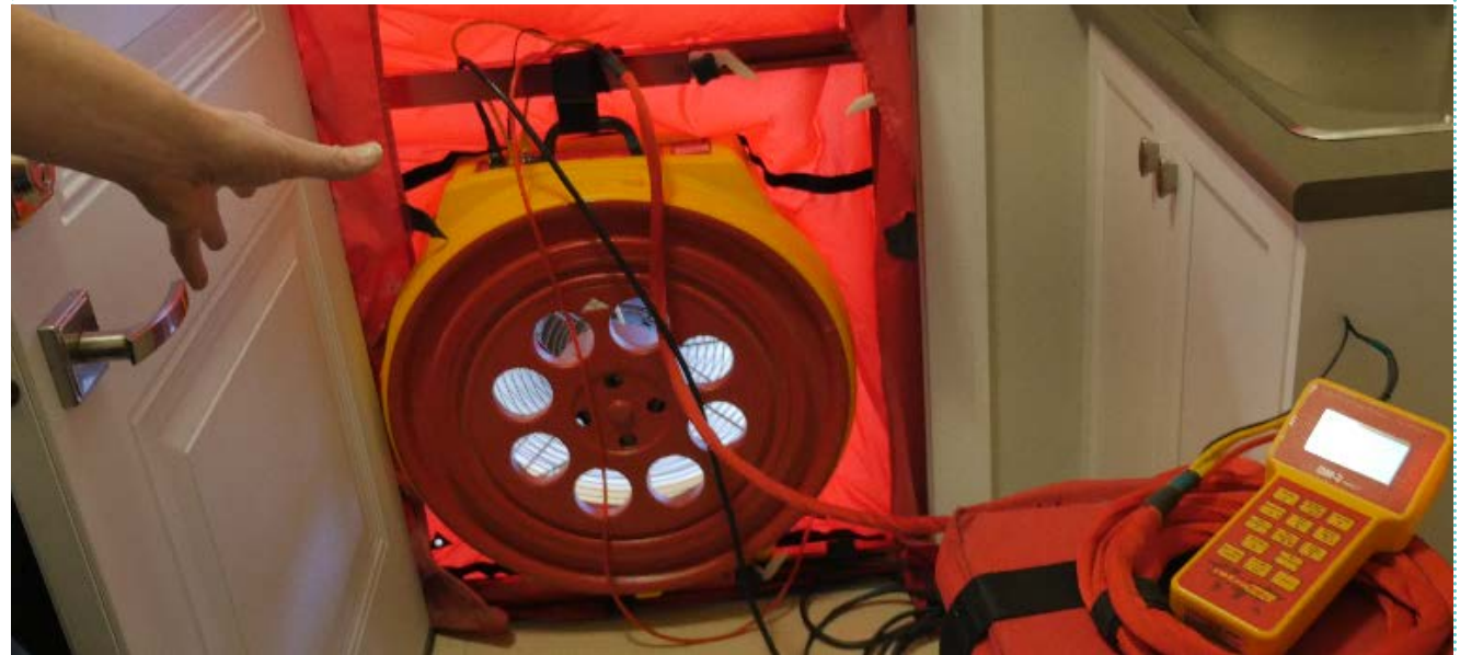
Figure 8: Blower door test in action
